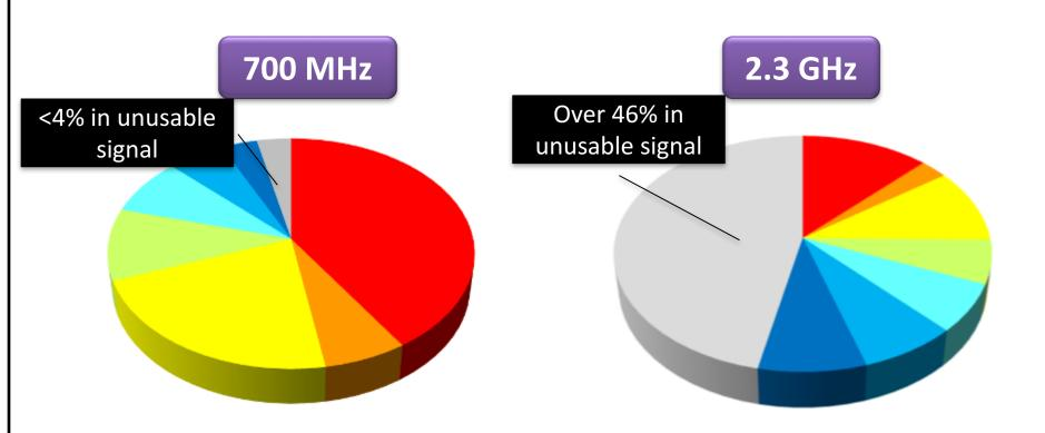
The 700 MHz coverage from the 25 sites estimates to cover over **96%** of the area of area of interest with at least QPSK. The 2.3 GHz estimates to serve just over **53%** of the area to the same signal level.
